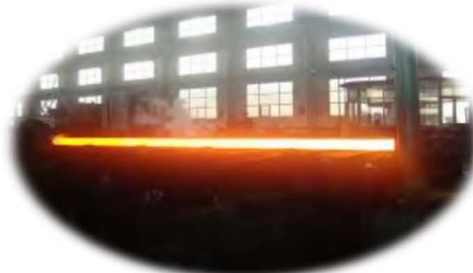
PIPE HOT-EXPANDING LINE
